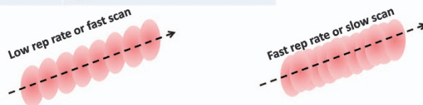
Figure 1 Schematic illustration of 3D photonic inscription where the waveguide is formed by increasing the local index of the material. The table shows how optical pulse energy, pulse repetition rate, and waveguide scan speed are adjusted to optimize the quality of the inscribed waveguide when the pulse width is held constant. Depending on the combination of laser repetition rate and mechanical scan rate, the material modification regions formed by each pulse will overlap by varying amounts. 3D, three dimensional.
