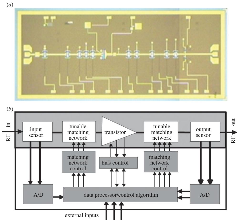
**Figure 7.** (a) Optical image and (b) block diagram of RF MEMS integrated with a GaAs amplifier to create a tunable broadband RF amplifier. In this iteration, the control circuitry (white box) was off-chip. (Online version in colour.)
