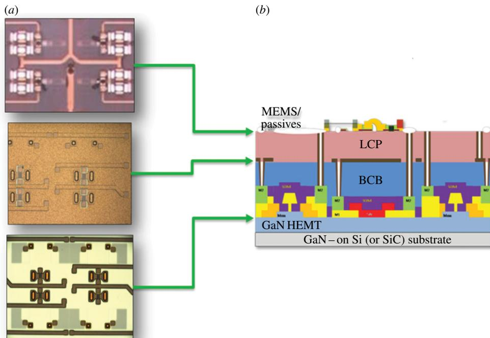
**Figure 8.** Schematic cross section (b) and optical images (a) of different layers of three-dimensional, integrated RF MEMS on GaN on silicon HEMT. (Online version in colour.)
