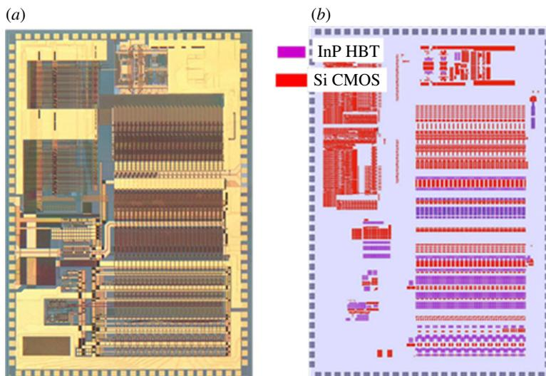
**Figure 4.** Optical image of completed COSMOS DAC-containing on-chip calibration circuitry (a) and CAD drawing showing intimate intermixing of InP HBTs and Si CMOS enabled by our integration approach (b). The circuitry in the upper left-hand corner is the on-chip calibration circuitry. (Online version in colour.)
