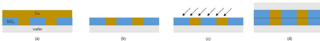
Fig. 15 DBI technology process, (a) form Damascus grooves, and electro-coppering.
