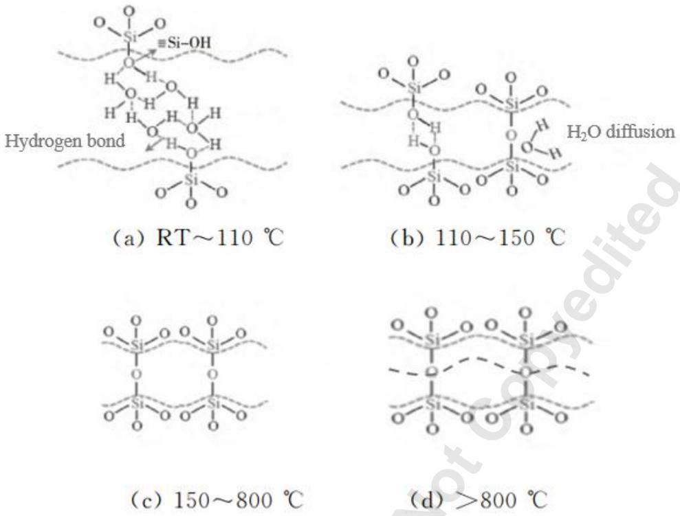
Fig. 11 Classical four-stage mechanism model of hydrophilic bonding [66]
