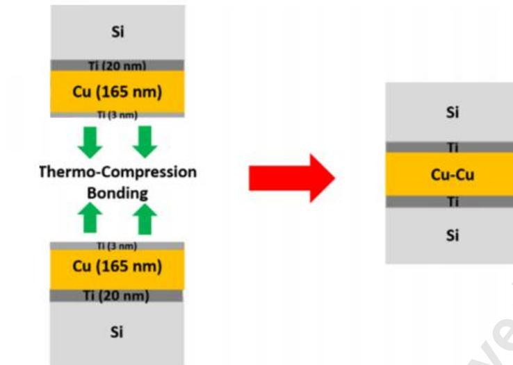
Fig. 8 Cu-Cu bonding mechanism of Ti passivation layer, Cu diffuses towards the bonding interface and forms diffused copper at the bonding interface [54]
