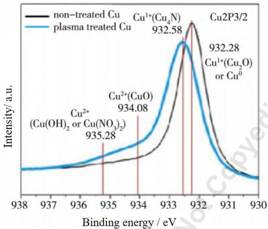
Fig. 20 XPS map of Cu surface after Ar and N<sub>2</sub> two-step plasma treatment, the XPS
