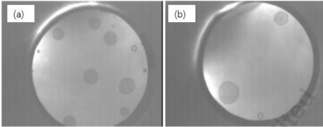
Fig. 13 Infrared transmission images of (a) without 29% ammonia treated and (b) 29% ammonia treated, the images show the bond rate of wafers treated by ammonia reached over 95% and the bonding strength reached 7.2MPa, while the bond rate of wafers treated without ammonia was only 80% and the bonding strength was only 3.1MPa<sup>[68]</sup>
