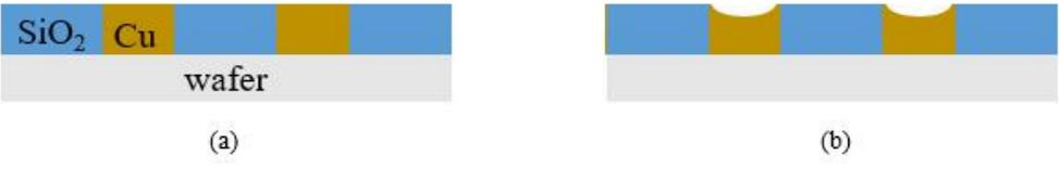
Fig. 16 chemical mechanical polishing (a) normal CMP and (b) dishing
