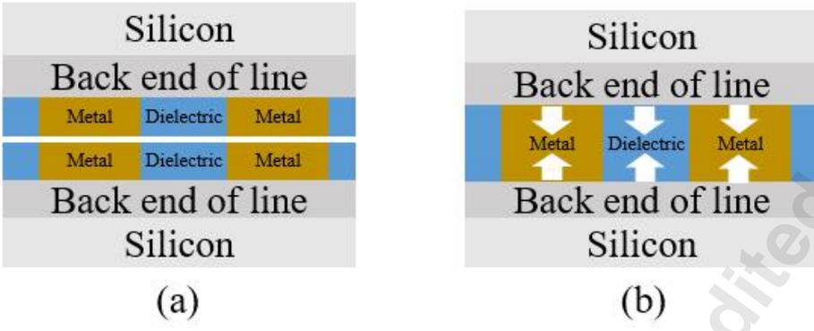
Fig. 1 Schematic of hybrid bonding (a) Dielectric material and embedded metal to be bonded (b) Dielectric material and embedded metal forming an interconnection after hybrid bonding
