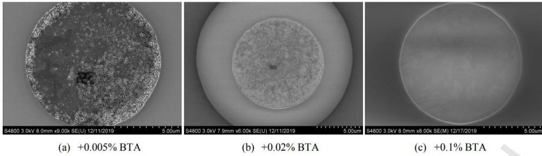
Fig. 17 galvanic Corrosion degree of different concentrations of BTA (a) 0.005% BTA.
