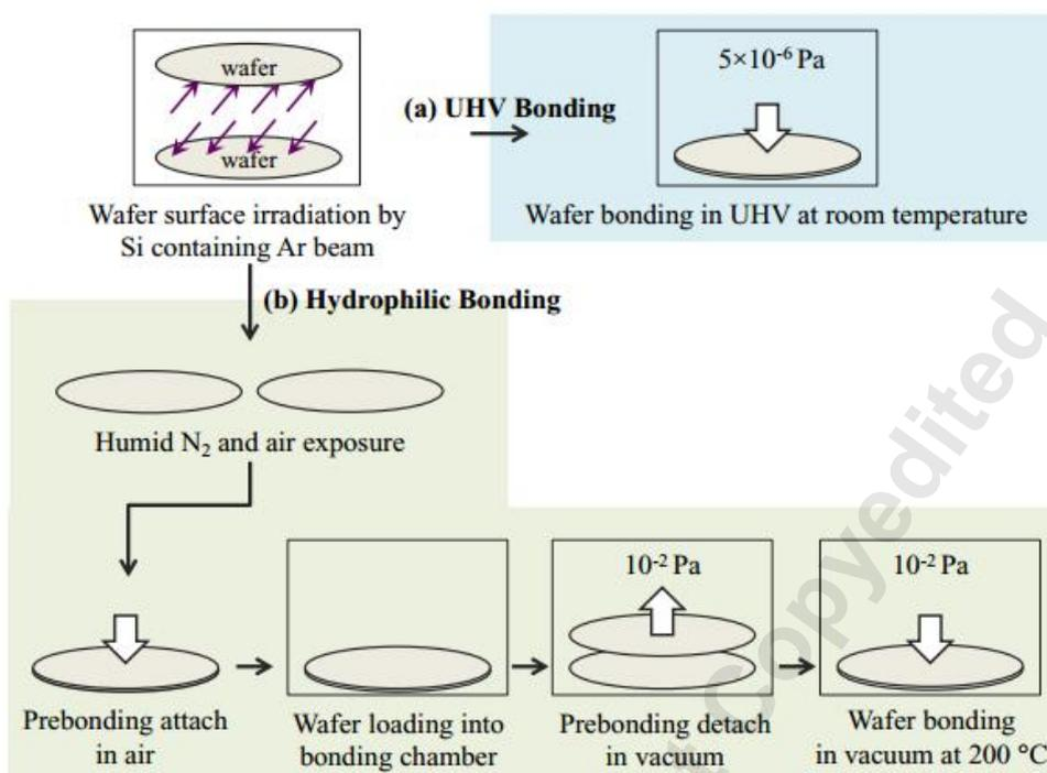
Fig. 19 Surface activation bonding process flow a) Direct bonding under ultra-high vacuum b) pretreatment - pre-bonding - separation - final bonding process [73]
