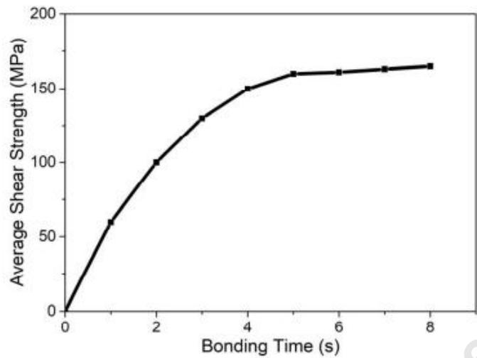
Fig. 7 Average shear strength vs bonding time for bonding pressure: 250 MPa and bonding temperature: 240 °C [47]
