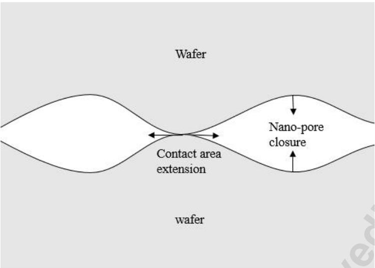
Fig. 12 Bonding contact model considering the surficial characteristics [67]
