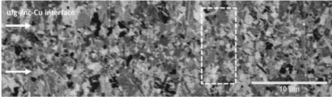
Fig. 5 SIM image of the overall interface of nc-Cu sample, SIM image show nc- Cu can be well bonded by thermo-compression bonding at the temperature of 250°C under the pressure of 10 MPa at the vacuum of 0.05 Pa for 60 min <sup>[45]</sup>
