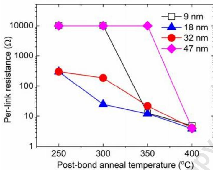
Fig. 18 Per-connection resistance as a function of post-bond annealing temperature for 4 different inter-die Cu-Cu gap heights [72]
