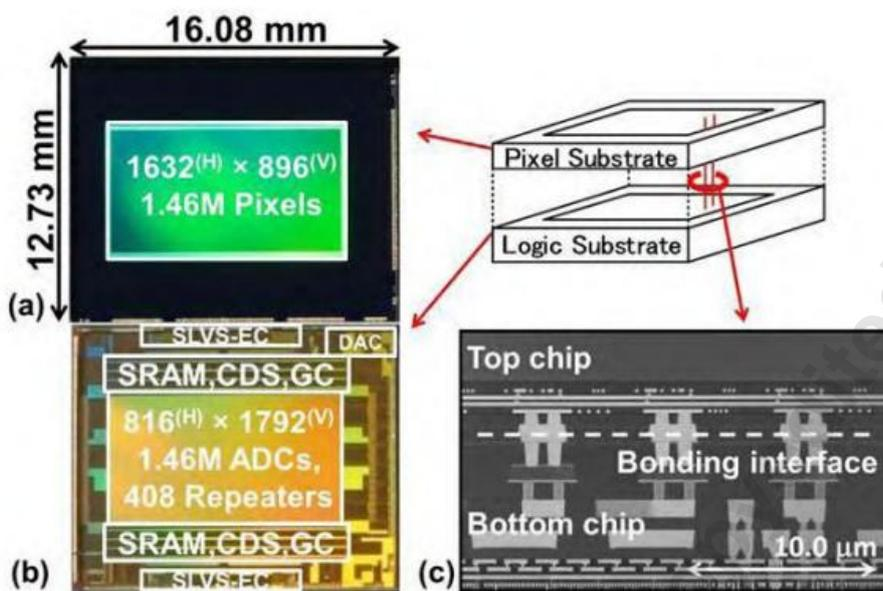
Fig. 2 Schematic of the connection of 90 nm CIS chip and 65 nm logic chip using SONY's hybrid bonding technology (a) CIS chip (b) logic chip (c) hybrid bonding cross section diagram <sup>[26]</sup>
