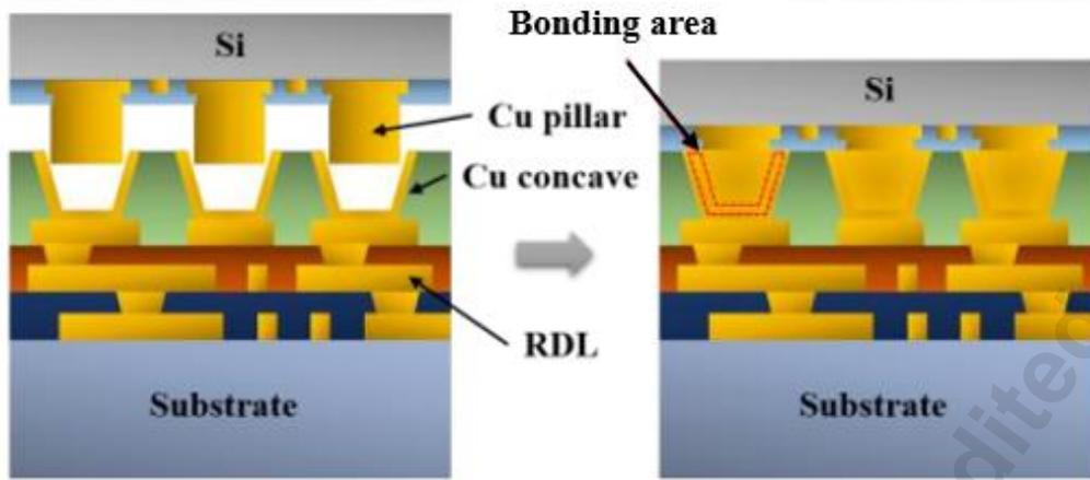
Fig. 6 Schematic of pillar-concave bonding, the protruding structure of Cu is inserted into the concave structure of Cu<sup>[46]</sup>
