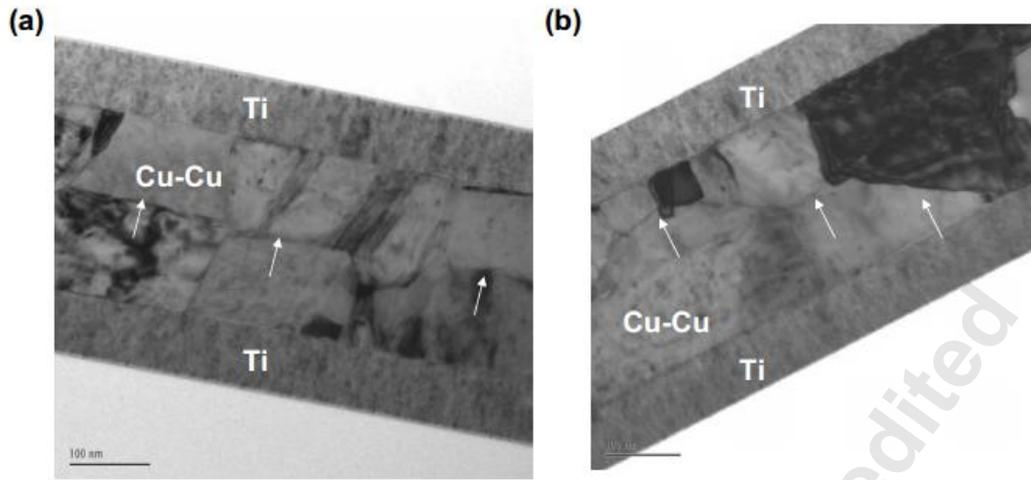
Fig. 9 TEM micrographs of bonded Cu layers, the bonding interface without passivation protection was still obvious, and under the protection of passivation layer, the bonding interface showed a clean bonding morphology. (a) without SAM passivation (b)with SAM passivation and desorption prior to bonding <sup>[57]</sup>
