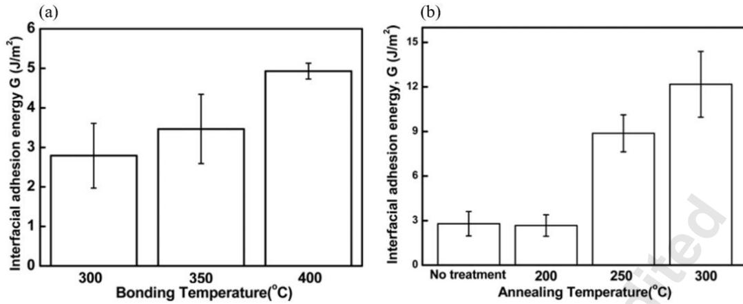
Fig. 3 (a) Changes of the interfacial adhesion energy between Cu-Cu bonded layer with bonding temperatures of 300°C, 350°C, and 400°C for 60 min without annealing treatment (b) Changes of interfacial adhesion energy between Cu-Cu bonded layer with post-annealing temperatures at 200 °C, 250°C, and 300°C for 60 min<sup>[33]</sup>
