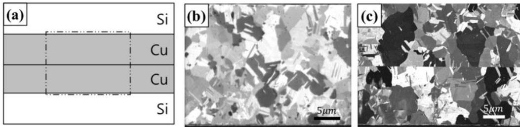
Fig. 4 HD Cu can be well bonded by the method of thermo-compression bonding, while the normal Cu bonding interface was still obvious under the same bonding conditions (a) Scheme of the Cu-Cu direct bonding. Vertical FIB images of the Cu-Cu direct bonding interface with (b) high defect density Cu and (c) normal Cu [44]
