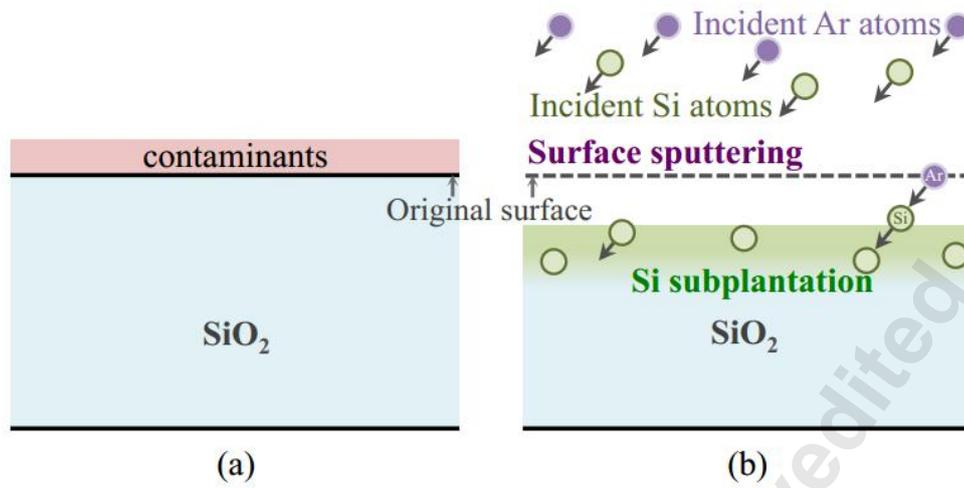
Fig. 14 Schematic representation of the Si-containing Ar beam irradiation on SiO<sub>2</sub> surface: (a) before irradiation and (b) after irradiation<sup>[69]</sup>
