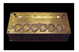
1642 – Pascal built a mechanical calculating machine
