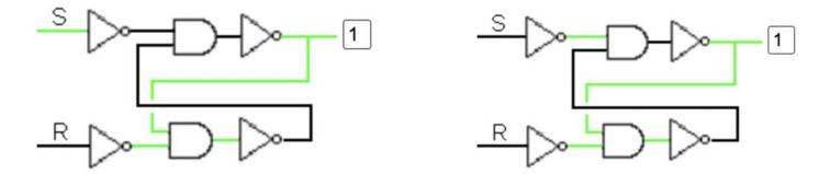
• a current burst on the Reset wire produces no output current
