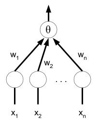
$$\begin{array}{l} \text{if } \Sigma_{w_i x_i} > = \theta, \text{ output } = 1 \\ \text{if } \Sigma_{w_i x_i} < \theta, \quad \text{output } = 0 \end{array} \end{array}$$
