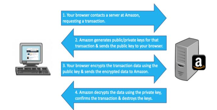
public-key encryption is also used whenever you surf the Web with https:// or use a secure Wi-Fi connection
