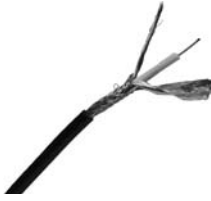
Figure 3-9 An example of coaxial cable
