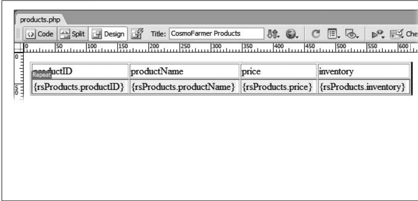
Figure 23-11: Although the Dynamic Table tool creates a table that displays multiple records, you see only one table row’s worth of dynamic data. The Repeat tab that appears above the row indicates that this row will repeat, once for each record in the recordset. To see the effect, use Live Data view as described on page 812).
