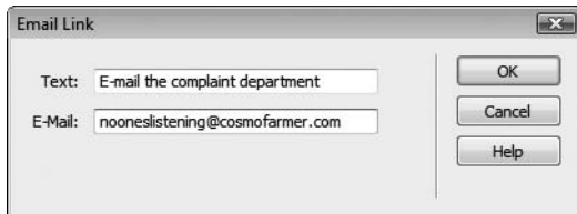
Figure 5-9: The Email Link dialog box lets you specify the text that appears on the Web page and the email address for a mailto link. You can also select some text you've already added to the document and click the Email Link icon on the Objects panel. The text you selected appears in the Text field in this dialog box.
