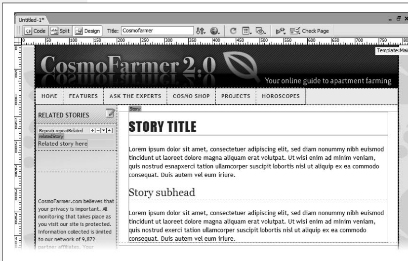
Figure 19-22: In template-based pages, blue tabs identify editable areas of the page, and the yellow tab at the top right lists the template’s name. Notice that the repeating region has small control buttons (+, -, and up and down arrows) and that one of the optional regions—the “Editor’s Selection” graphic—is invisible. (Remember, you deselected the “Show by Default” option for this region.)
