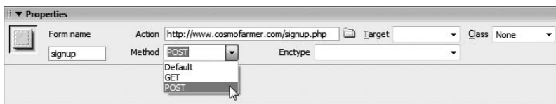
Figure 11-3: You'll generally want to use the POST method of sending data to the server. See step 7 for more details.
