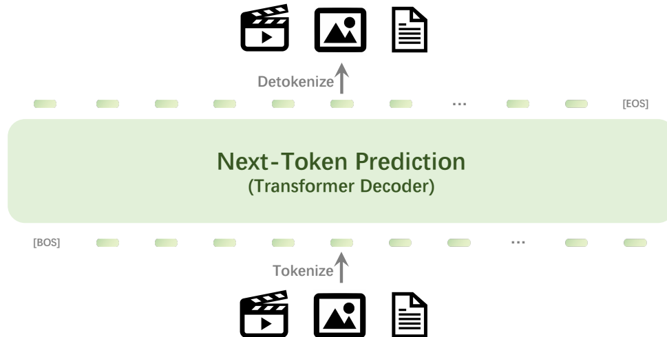
Figure 1: Emu3 is trained to predict the next token with a single Transformer on a mix of video, image, and text tokens. Emu3 achieves state-of-the-art performance compared to well-established task-specific models in generation and perception tasks.
