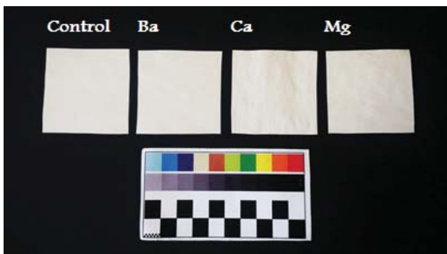
Fig. 1. Treated samples after accelerated aging compared to aged control sample.
